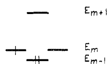
Figure 3. Typical electronic configuration for which a quartet state may be the lowest excited state.
